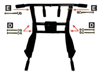
The screw fixing process suggests that each screw hole should be looselyfixed on the top and then all the screws should be loosely fixed before they are tightened together SO that themain frame is installed.
