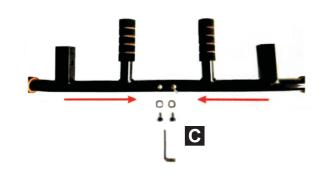
Firstly, butt the left and right multifunctional connecting tubes and then fix the alignment screw holes loosely. If fixed tightly, it will affect the subsequent installation smoothly!
