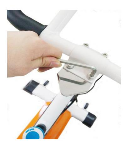
5). Take out the armrest. Put it at the screw holes, stack up the washer and cylinder screw to fasten them with 6-side spanner.
