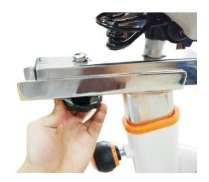
3). Take out the cushion and place it at the cushion seat. Adjust the angle and fasten them with screws. Loosen the brake and adjust the cushion to the appropriate height. Fasten the brake and seats. (You can adjust the cushion seat backwards and forward by loosening the plumhead bolts to a comfortable situation. Ensure you tighten the plumhead bolt after adjustment.)
