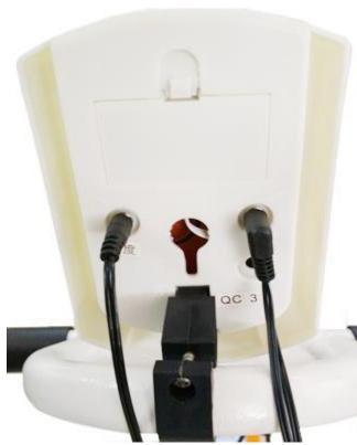
7) Fasten the electronic watch into the slots and connect the cables as illustrated in the picture. (Double wire with right Pulse and single wire with left sensor.
