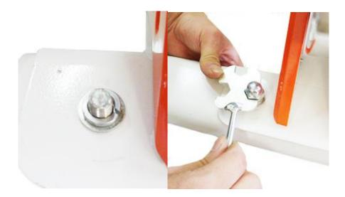
1) Connect the front tube with the frame and install the plain washer 10 (no.3) to the bolts and put on the cover-shaped screws. Use open spanner to tighten them. Assemble the back tube is the same way.
