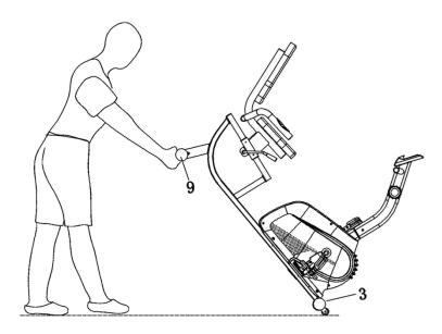
Hold the **Rear Stabilizer (No. 9)** and lift the bike until wheels on the **Front Stabilizer (No. 3)** touch the ground. Now you can wheel the bike to the desired location.
