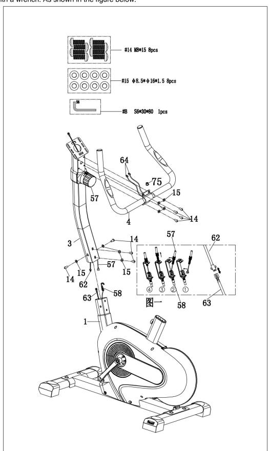
Step 3: please turn out the screws (44) on the digital watch (61), and then you will attach the hand pulse sensors (64), hand pulse wire (62), and then install the electronic form digital watch (61) and lock it with the screws (44). This is shown in the figure below.
