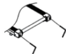
**Note:** The running belt cannot be adjusted too tightly. This will pull the running belt, increase the pressure of the front/rear drum, and damage the drum bearings, resulting in damage to the treadmill. Only adjust the running belt so that it does not slip during operation.
