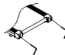
**Note:** The running belt cannot be adjusted too tightly. This will pull the running belt, increase the pressure of the front/rear drum, and damage the drum bearings, resulting in damage to the treadmill. Only adjust the running belt so that it does not slip during operation.
