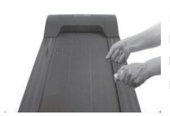
Pull up the running belt, then put silicone oil onto the running board. Start the machine and let it run for three minutes without loading. It is best to do this after every 30 hours of use, ensuring parts are maintained.
