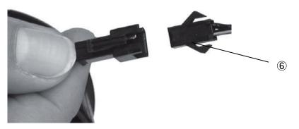
4.Connect the computer to the device using the plug ⑥ without bending or breaking the pins inside.
