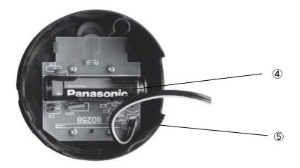
3.Insert the supplied battery into the battery compartment ④ in the computer casing ⑤:
