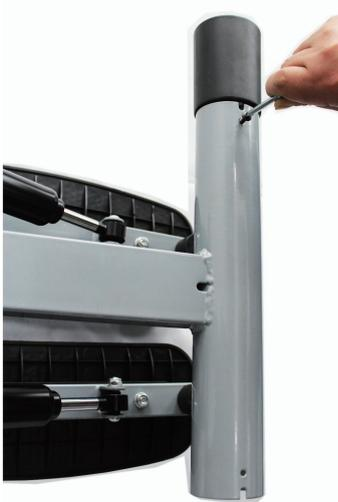
2. Insert the bushing(13) to the front tube of the main body.
