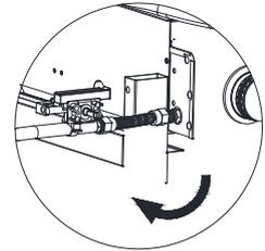
EN\_Use wrench to tighten the screw
