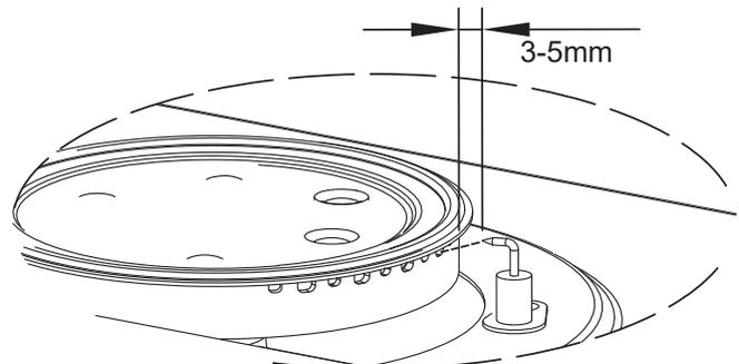
EN\_After assemble side burner,insert ignition wire into ignition pin
