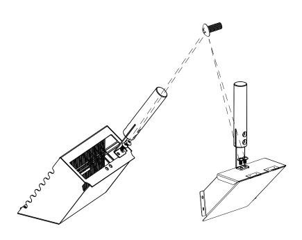
Step 2. Attach the hopper and wood box to the back of the body.
