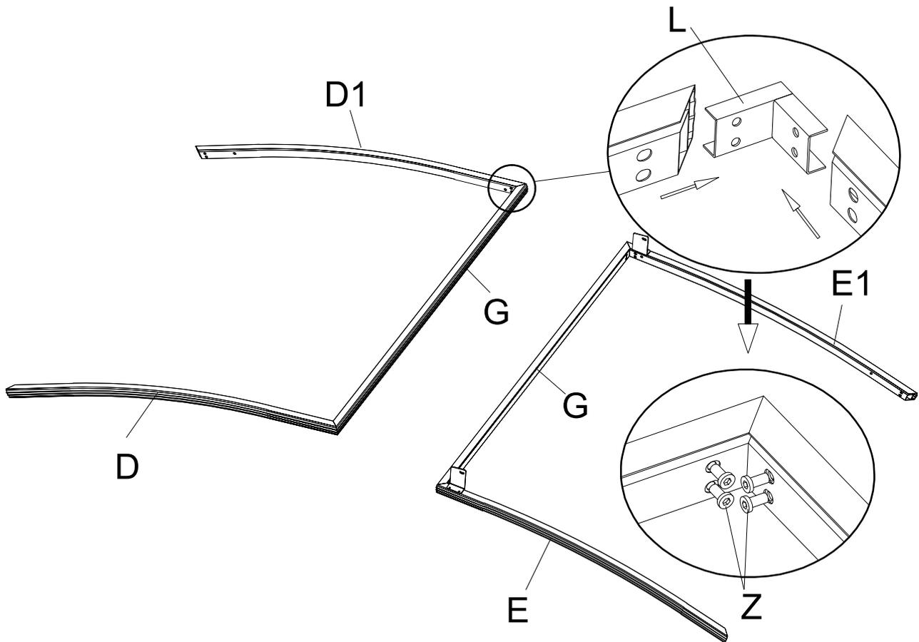
The tube (G) and D1 is connected with the L-shaped connector (L) and fixed with the screws (Z).
