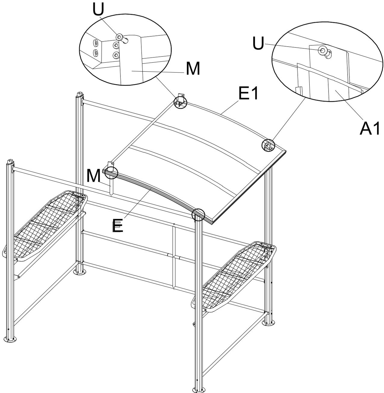
Place the assembled PC board assembly on the tube as pictured. Use the screw (U) to connect the tube E/E1 with the leg. Connect with the M bracket with the screws (U).
