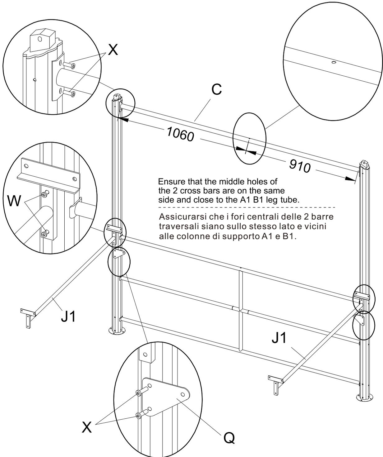
Ensure that the middle holes of the 2 cross bars are on the same side and close to the A1 B1 leg tube.
