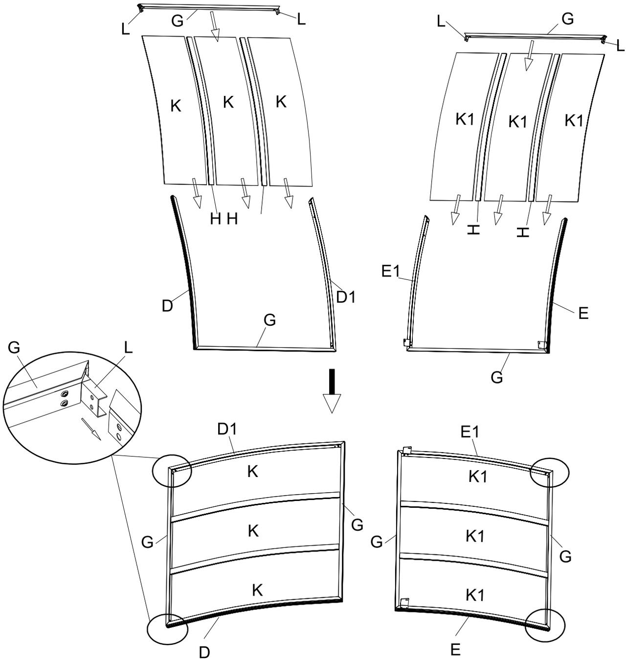
Put the PC board (K) into the tube(D1) and (G),install each of the other PC board and tube in turn. Repeat the above steps to the PC board assembly.
