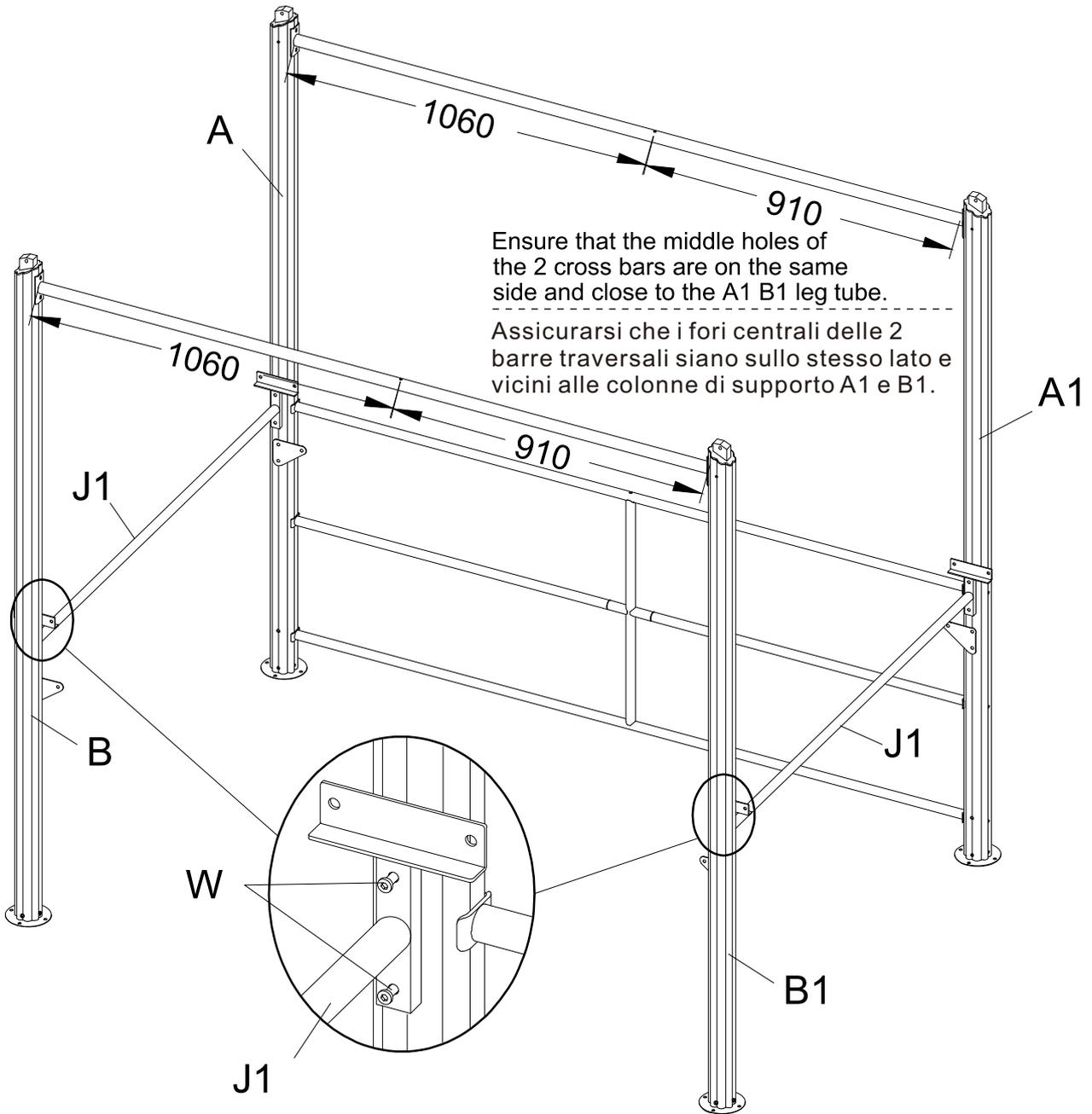
Place the leg(B) and leg B1 in place to connect the cross bars (J1) with screws(W)
