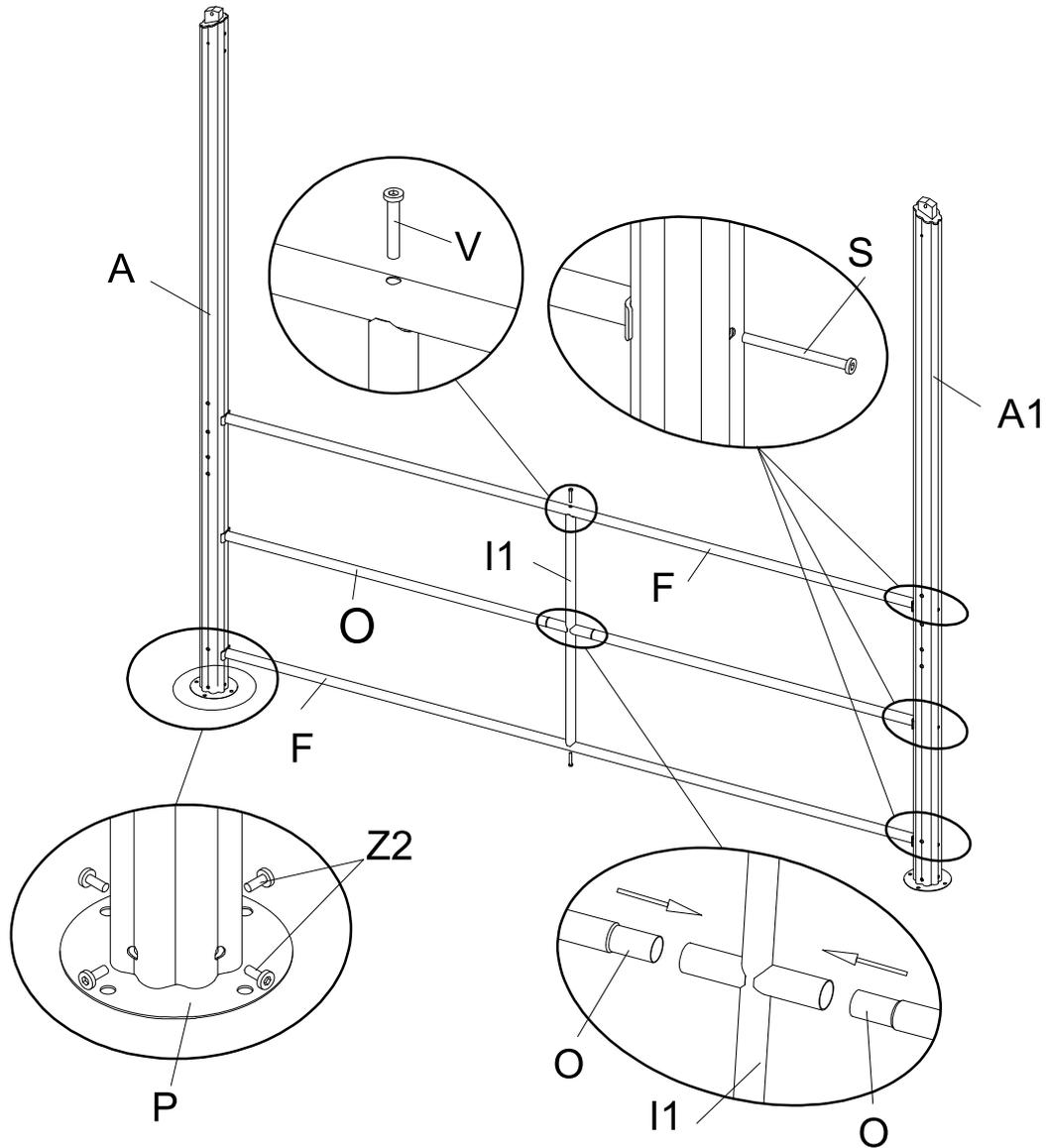
Put the leg (A) on the foot pad (P) and fix it with 4pcs screws (Z2), Repeat the above steps for the leg(A1).
