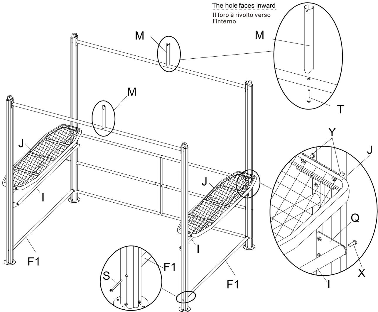
Fix the tube (F1) at the bottom of the leg with screw (S)
