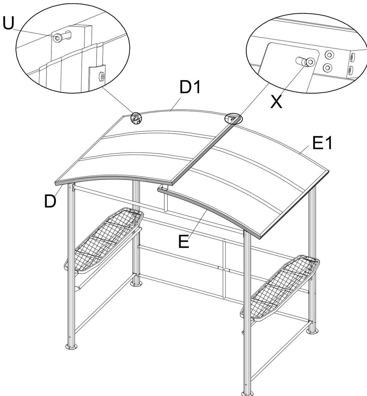
Place the other assembled PC board assembly on the top as pictured. Use the screw (U) to connect the tube D/D1 with the leg, then connect D and E ,D1 and E1 with the screw (X).
