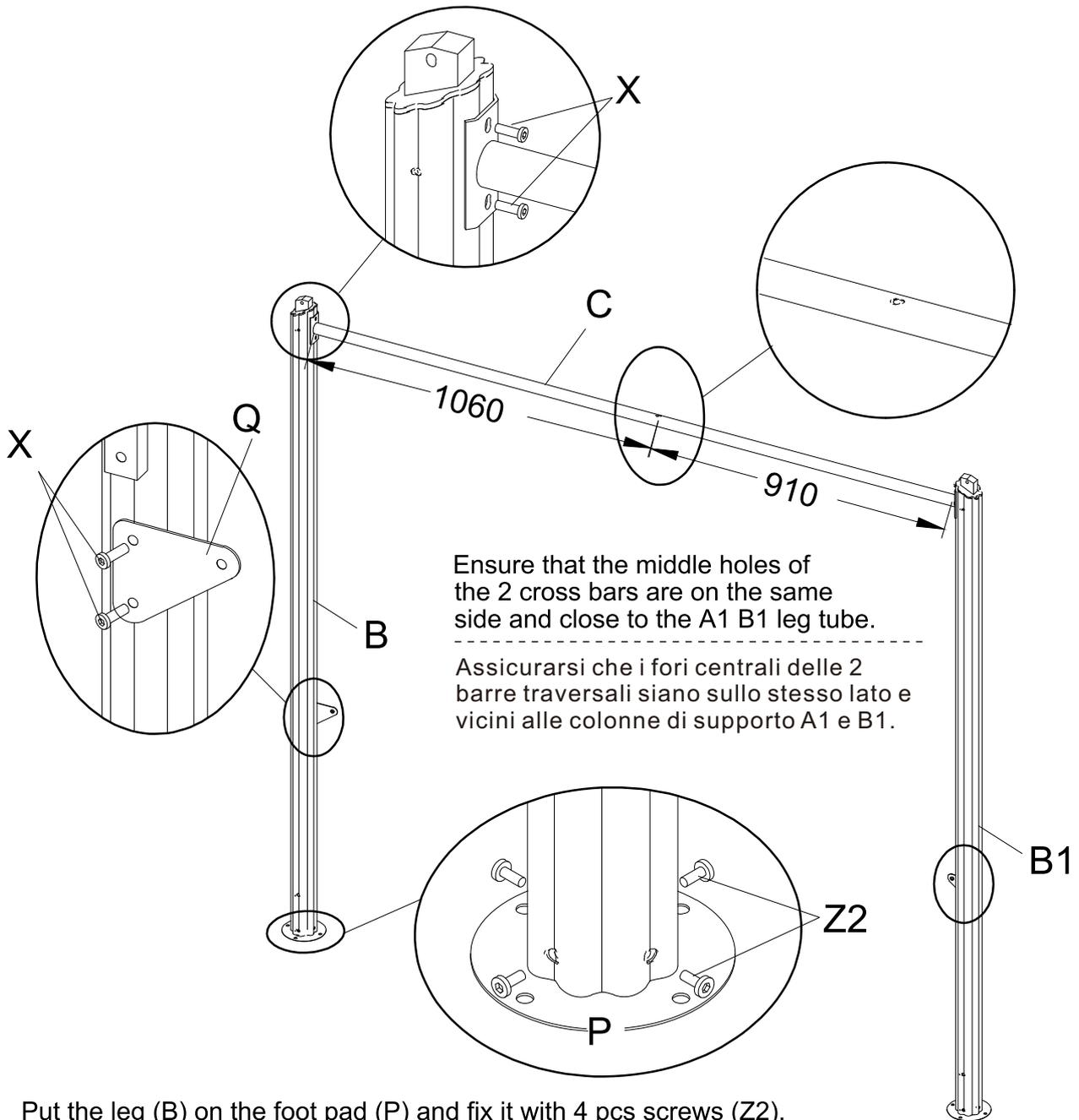
Ensure that the middle holes of the 2 cross bars are on the same side and close to the A1 B1 leg tube.
