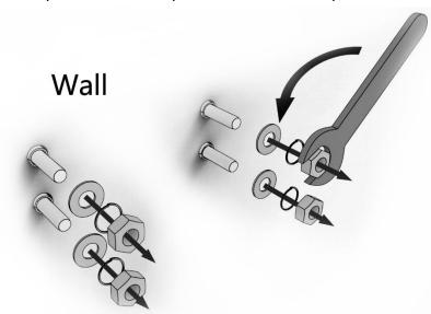
**Step3:** Installer the heater on the wall
