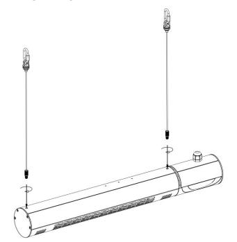
Step 2: loosen the safe lock and hand on the ceiling.
