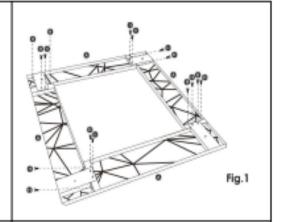
Step 2) Attach Frame Support Parts (C) to Legs (B) by using Bolts (H). Tighten all hardware accordingly with an Allen Wrench (J) (provided) and adjustable wrench until all pieces fit together securely. Turn the assembled fire pit frame over so that it sits securely (legs down) on a flat surface
