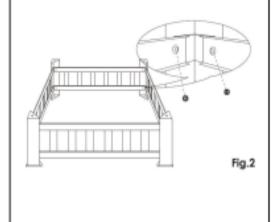
**Step 3)** Attach Legs (B) to Top Frame (A) with Bolts (H) Hand tighten (View Fig.3)! [4 x (H)]
