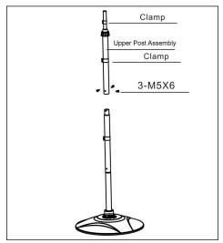
4.Put the small cord support to the top tube and fix the heater head to the top tube by the plastic screw in the heater head
