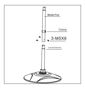
3.Screw out 3pcs M5\*6mm screws in the middle tube and put the cord support to the top tube before fix the top tube.
