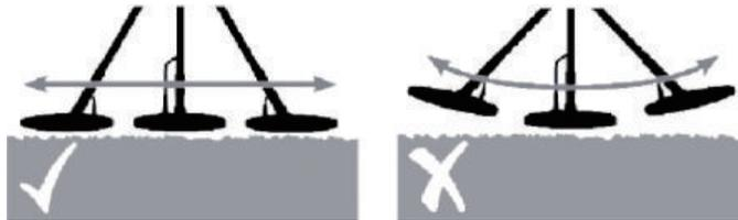
Sweep slowly hurrying will cause you to miss targets. It's better you sweep the search coil from side to side in an arc line of 3 inches motion and keep the search coil parallel with the ground.
