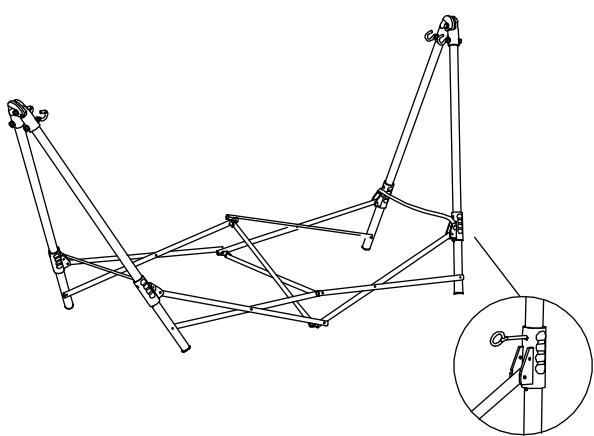
**EN\_2.** Insert the pin (4pcs) into the hole on the lower plastic frame slider. Make sure that the pin is fully inserted into the leg.
