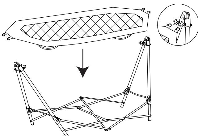
**EN\_3.** Connect all 4 loops on the hammock bed to the hooks at both ends of the frame.
