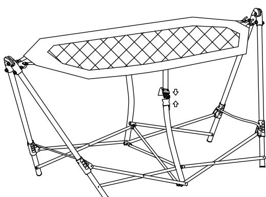
**EN\_4.** Connect the anti-tip buckles on both sides of the hammock with the buckles on the frame. Otherwise, it may cause injury.
