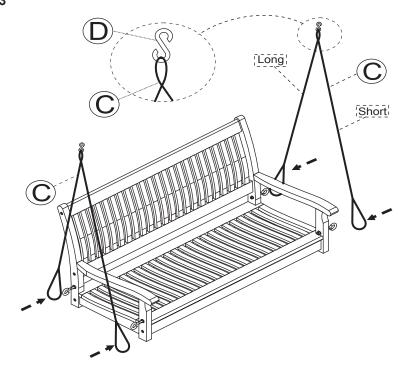
Tightly secure the Rope (C) to the Hooks (B) as indicated, making sure that the short side of the rope faces forward.
