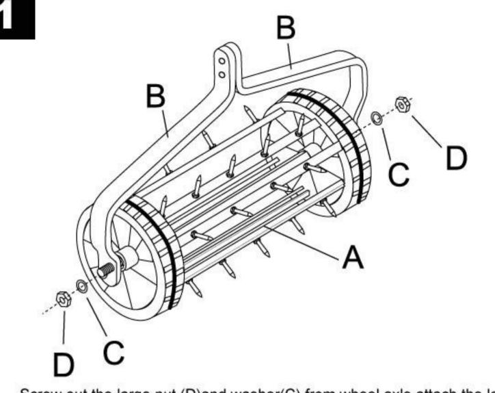
Screw out the large nut (D)and washer(C) from wheel axle, attach the left and right frame(B) to the main unit(A), and across the wheel axle push on the large washer(C), large nut (D) onto two side, Ensure fixings are secured tightly and correctly.
