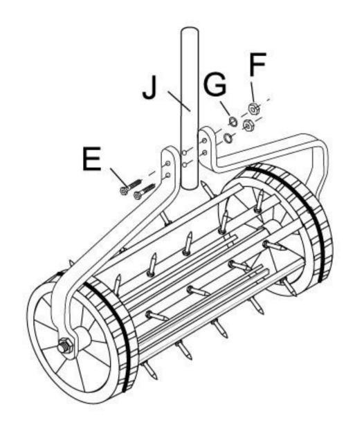
Using (E),(F) and (G) parts screw the left and right frame (B) to the tube(C) please sure to tighted all fixings securely.
