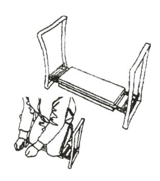
To fold the legs back together: Kneel on the seat and press the feathers together by pressing the small rod against the outer edge.
