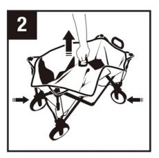
Pull the handle in the middle of the bottom to lift it up, the wagon will be folded, and the corners on four sides of the wagon will be leaned inward against one side with one hand.
