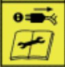
Always disconnect the machine from the power mains before cleaning inspecting, repairing or when it is damaged or tangled.
