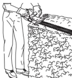
5. If the blades do become jammed, release the trigger switch and allow the blades to stop. Remove the battery pack before attempting to remove the obstruction.
