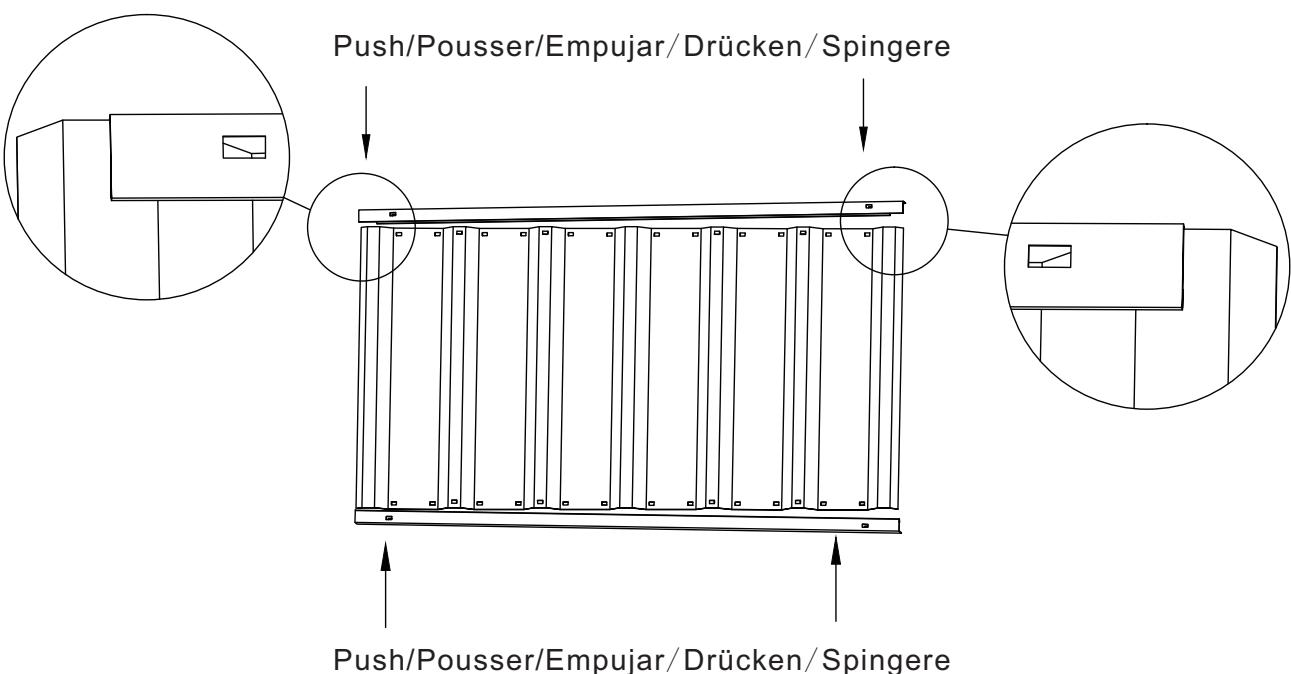
**EN** Install the card frame on the sheet by one side to the other side; make sure the card frame connected with the sheet completely.
