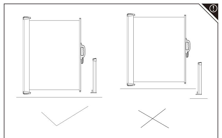
Warning: When mounting the awning, keep the cassette part and stand column on the horizon, or the fabric will deformation and difficult to open and close.
