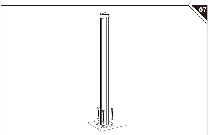
7. Make the left bottom hole of stand column and the hole on the floor alignment, and tighten them with M8x75 hexagon tapping bolt.
