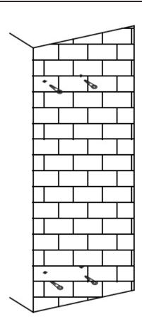
$2. Insert\ one \phi 10x 50mm\ plastic\ expansion\ tube\ in\ each\ of\ holes.$
