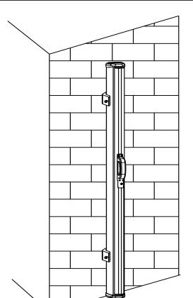
4.Insert the cassette part into the bracket, tighten the flat fillister head screw M6x16mm with Hexagonal spanner CR-V5mm
