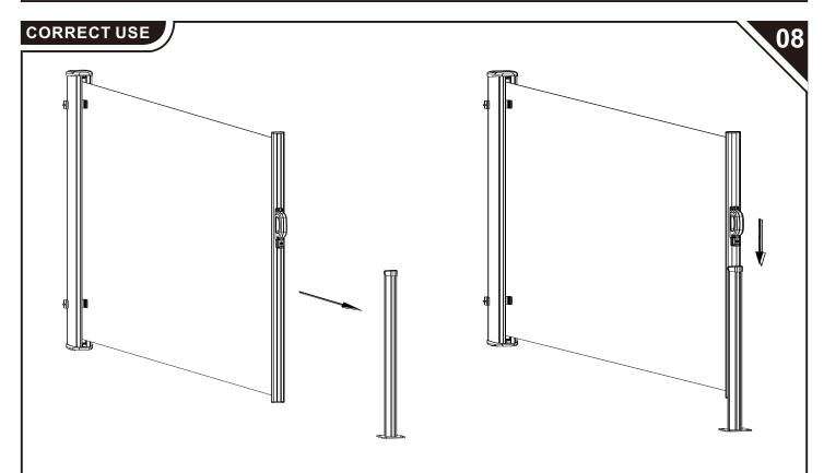
1.Keep the front bar upright, hold the handle and pull it over the column. Hold the handle tightly, rotate it 90 degrees, align the side of the front rod with the groove of the column and put it in, so that the main shaft of the handle can be clamped into the groove. See the figure below for details
