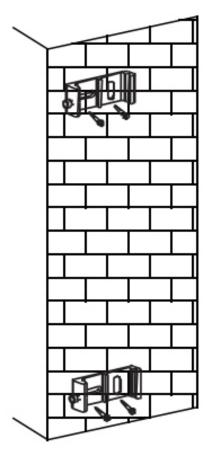
3. Fix the bracket with M6x60 hexagon tapping bolt
