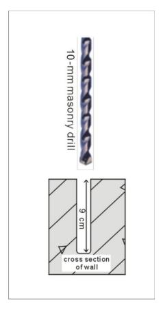
5.Drill four 10mm diameter holes on the floor in the size as the following picture shows
