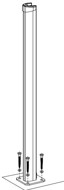
7. Make the left bottom hole of stand column and the hole on the floor alignment, and tighten them with M8x75 hexagon tapping bolt.
