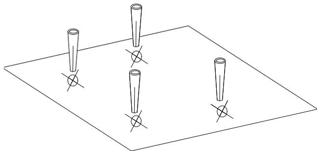
6. Insert one  $\text{Ø}10 \times 50$  mm plastic expansion tube (4 pcs) in each of holes
