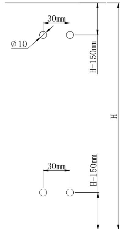
2. Insert one  $\text{Ø}10 \times 50 \text{ mm}$  plastic expansion tube in each of holes.
