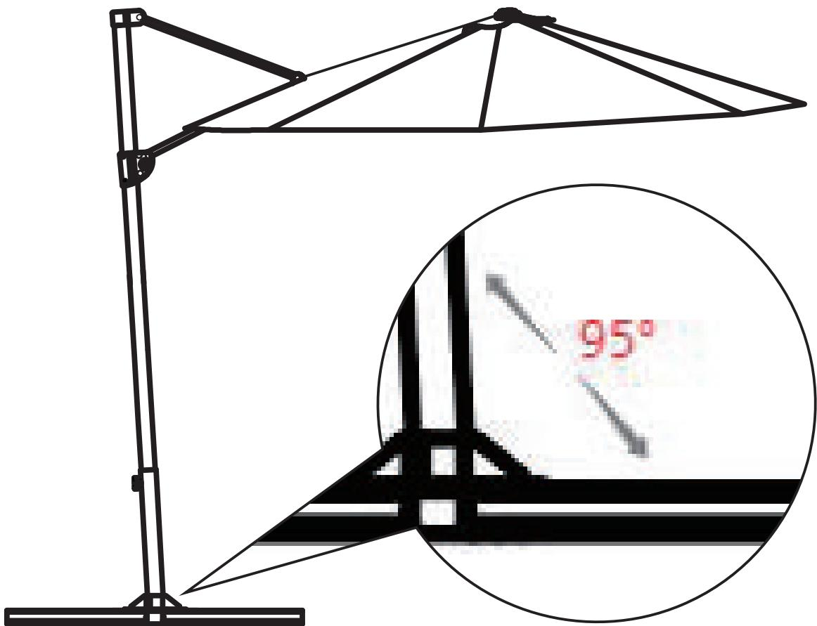
**EN** \_The structure here is specially designed to be inclined angle, the purpose is to enhance the strength of the umbrella base, please do not mistake the product as a defect.
