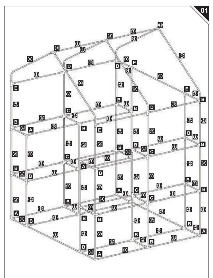
**ACAUTION:** Make sure the tubes are fully seated in the connectors before continuing.
