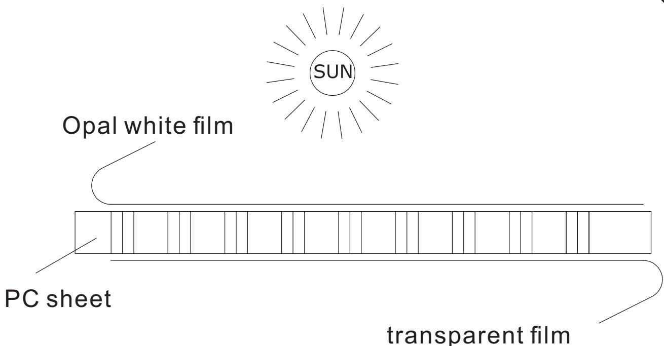
Two sides of PC sheet are covered with thin film, one side's film is transparent, another's film is opal white. The UV-protected side of the sheet is covered with opal white film and must face towards the sun.
