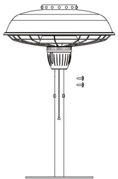
Step 3: Fix the power cord onto the slots.
