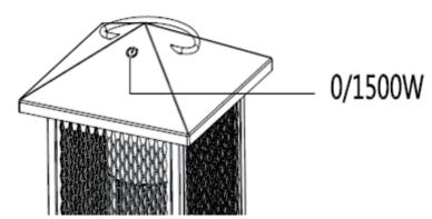
Press the switch to turn the heater on (1500W).
