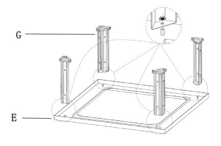
Step4. Put the panel (F) to the Leg (G), using M6\*20 bolt(AA) and M6 Nut(C-C), then tighten all nuts by Wrench (DD).
