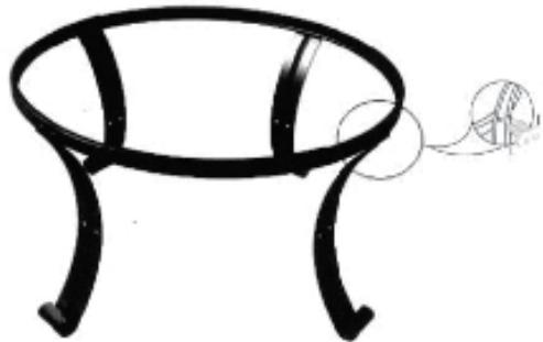
**Step 2)** Attach and tighten the small support ring to each leg, using bolts (I) and a nut (J). Fully tighten all bolts.
