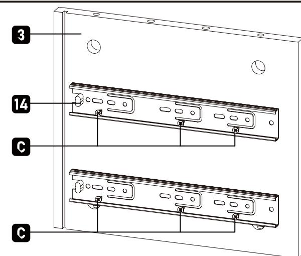
**EN:** By moving the middle slide and adjusting the position of it, you can use part C to fasten the outer slide to the board. Please pay attention to the orientation of the slide.
