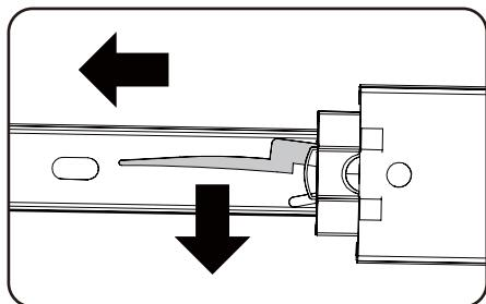
**EN:** Undraw the inner slide from the left side as shown and press the plastic limiter. Then pull out the inner slide.
