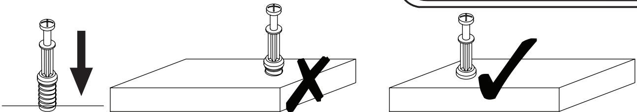
**EN\_QUICKFIT:** Tighten quickfit until shoulder is flush with panel. Do not overtighten or undertighten.
