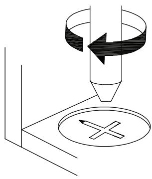
**EN**\_Turn cam lock clockwise to tighten.
