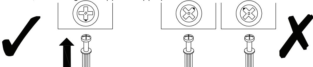
**EN\_CAM LOCK:** When fitting cam lock, ensure starting position is correct before you insert connecting quickfit.
