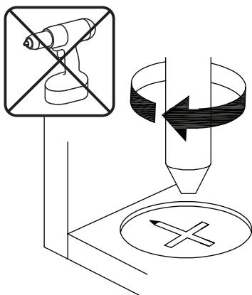
**EN**\_Turn cam lock clockwise to tighten.
