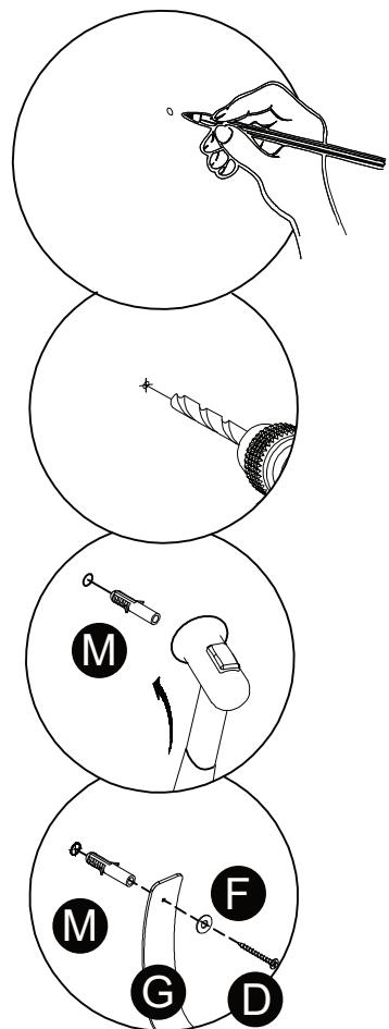
**EN** If it is a solid wall, please use expansion and self-tapping screws, if it is a wooden wall, only use self-tapping screws, please do not overtighten the screws
