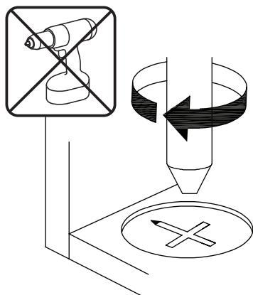
**EN**\_Turn cam lock clockwise to tighten.
