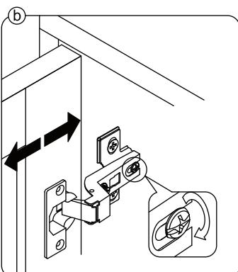
**EN** To adjust the gap from the door to the main frame turn the screw clockwise or anti-clockwise as needed.
