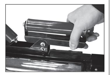
Push down the spring mechanism to tilt the V-shaped Rollers.
