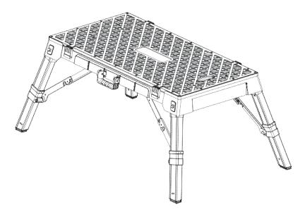
3. Remove the panel and turn it over, so the surface is facing up. Place it back onto the platform and refasten all four latches.
