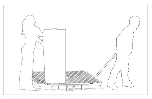
Two holes are provided on one end of the product for attaching a traction roper connecter when moving heavier objects.
