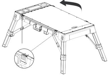
2. Open the four latches on the sides (two latches per side).
