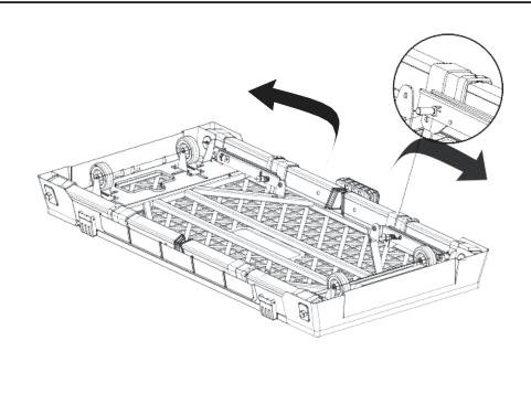
1. You must pull out the spring loaded locking pins when opening the legs, otherwise they can get damaged and may not open.
