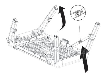
2. Pull each leg up and out – extend the hinged bracket until it locks in place.
