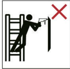
t) Do not carry equipment which is heavy or difficult to handle while using a ladder.
