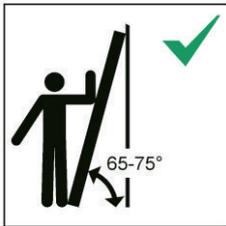
Correct erection angle (65°-75°)
