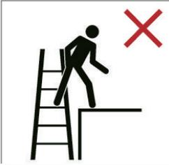
Do not step off the side of a ladder onto another surface
