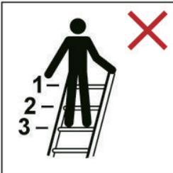
b) Do not overreach; users should keep their belt buckle (navel) inside the stiles and both feet on the same step/rung throughout the task;
