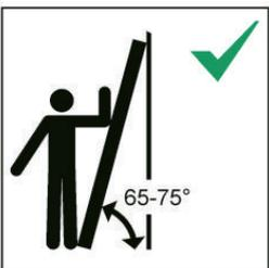
a) The ladder shall be erected at the correct position, such as the correct angle for a leaning ladder (65-75° angle of inclination, approximately 1:4) with the rungs or treads level and complete opening of a standing ladder;
