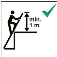
Ladders used for access to a higher level shall be extended at least 1m above the landing point and secured, if necessary. When the hinge ladder is used as access equipment for a higher level, the ladder has to be secured against unintentional sideways sliding.
