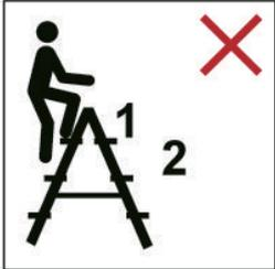
Do not stand on the top two steps/rungs of a standing ladder without a platform and hand/knee rail.
