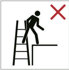
Do not step off the side of a ladder onto another surface
