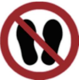
Any horizontal surface which looks like a platform on a standing ladder that is not designed for standing on (e.g. a plastic work tray) shall be clearly indicated on that surface, (only if necessary due to design of ladder).
