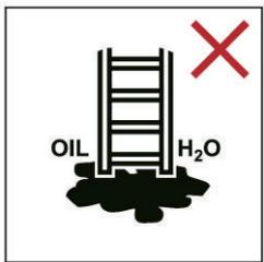
Do not erect ladder on contaminated ground
