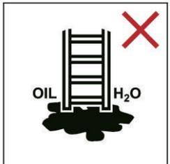
Do not erect ladder on contaminated ground
