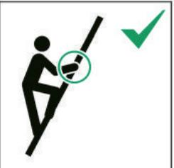
c) A leaning ladder should lean against a flat non-fragile surface and should be secured before use, e.g. tied or use of a suitable stability device;
