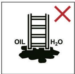
Do not erect ladder on contaminated ground
