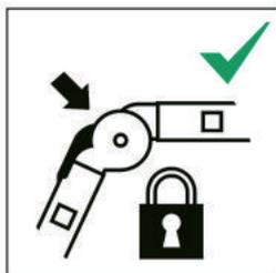
w) Ensure that the hinges are locked.
