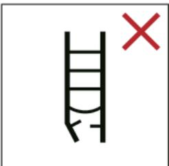
c) Inspect the ladder after delivery. Before every use visually check the ladder is not damaged and is safe to use. Do not use a damaged ladder;
