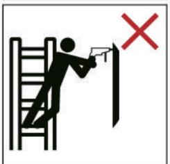
b) Do not overreach; users should keep their belt buckle (navel) inside the stiles and both feet on the same step/rung throughout the task;
