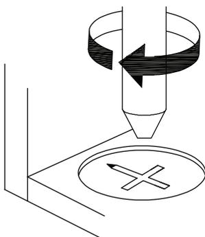
**EN\_**Turn cam lock clockwise to tighten.
