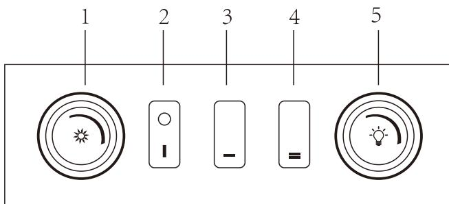
1. Thermostat control knob (**TEMPERATURE SETTING**): Adjust to maintain room temperature.
