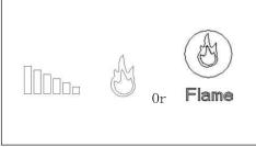
Under standby, press Flame button, the flame will be on at brightest. The charcoal set will be lit up and flicker automatically at a slow pace. Each time this button is pressed, the intensity of the flame decreases. There are five brightness levels you can cycle through including the OFF setting. Caution: When the heat is on, the charcoal set will keep lit-up if you turn off the flame.
