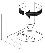
**EN** Turn cam lock clockwise to tighten.
