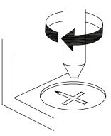
**EN** Turn cam lock clockwise to tighten.
