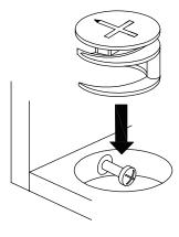
**EN** Quickfit head should be in the centre of the cam lock when the two panels are joined.
