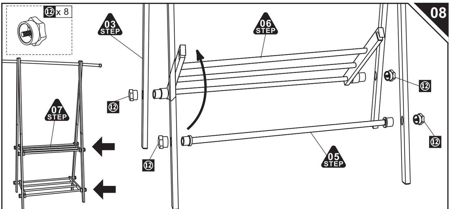
UK: Fix the part which is already finished in step three into the big hole at the bottom of two outer tubes , and tighten them with 12 lightly. After 5 and 6 are both finished fixing toally, tighten 12 with your strength tightly.
