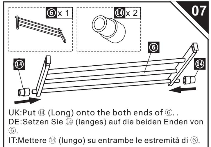
UK: Put 14 (Long) onto the both ends of 6 . .
