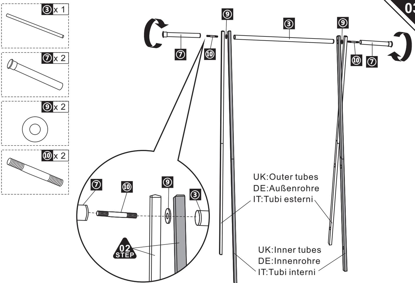
UK: Put ⑩ into the upper hole of tube ②. Put ⑨ between tube ③ and tube ⑦, then tighten tube ③ and tube ⑦ with your strength (another side is with the same way to fix). After finishing aboved steps, adjust two inner tubes to same direction. And two outer tubes to the opposite direction.
