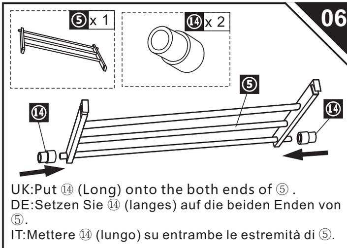
UK: Put 14 (Long) onto the both ends of 5 .
