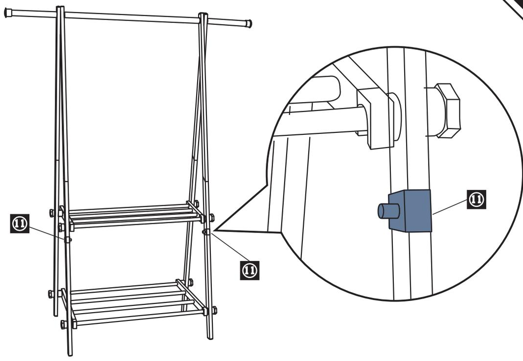
UK: Fix ① on the suitable place of two inner tubes, you can adjust the place of ① as you need when you fold the rack.
