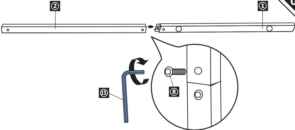
UK: Connect tube ① and tube ② with screw ⑧ as shown below.
